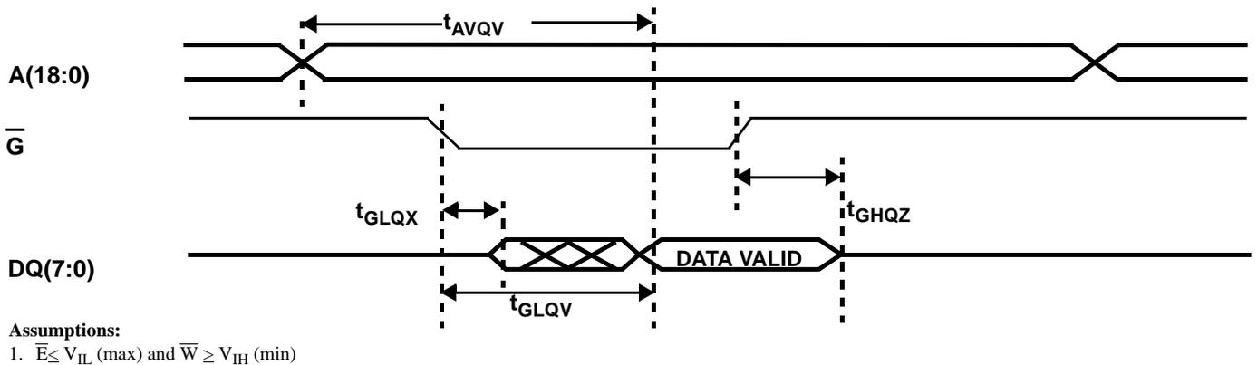
Figure 4c. SRAM Read Cycle 3: Output Enable-Controlled Access
