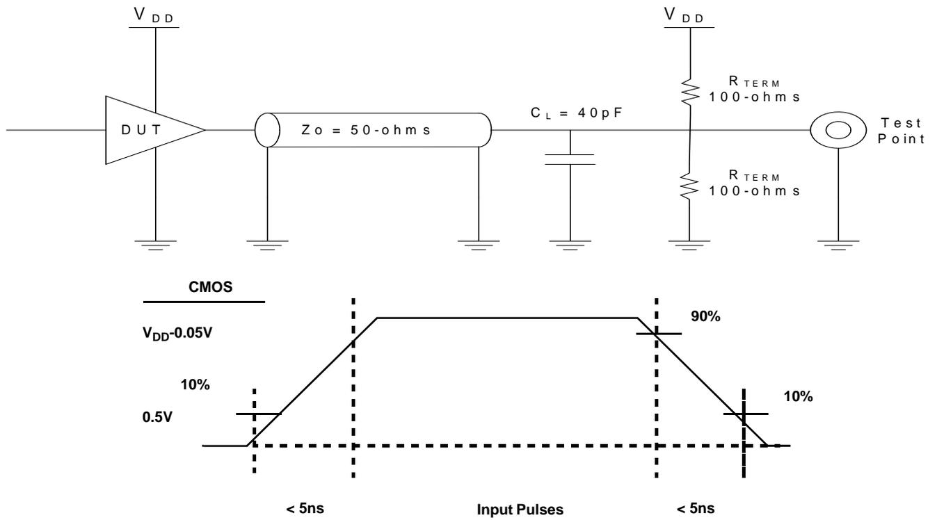
**Figure 6. AC Test Loads and Input Waveforms**
