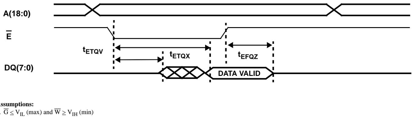
Figure 4b. SRAM Read Cycle 2: Chip Enable-Controlled Access
