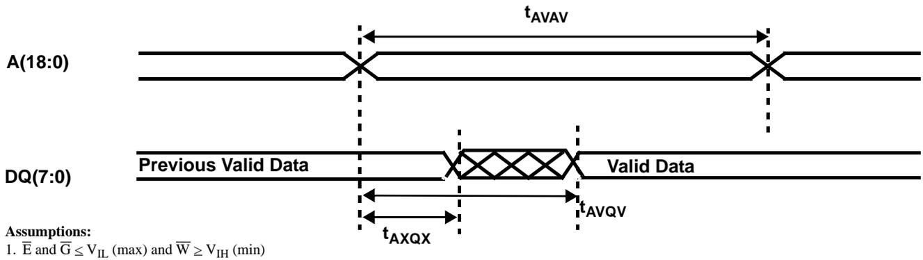
Figure 4a. SRAM Read Cycle 1: Address Access
