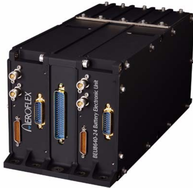
FIGURE 3 – Box Assembly, Li Battery Electronic Unit (BEU)
