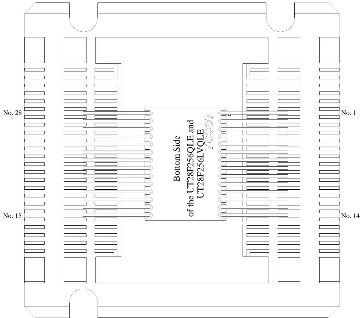
**Figure 1. Diagram of the UT28F256QLE and UT28F256LVQLE PROM 28-Pin Flat Pack in Carrier**
