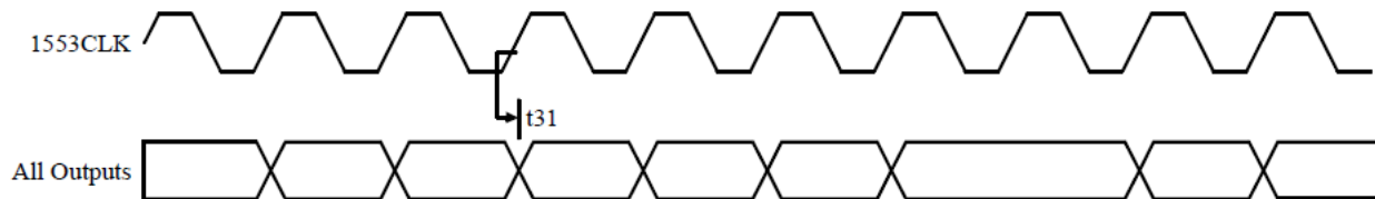
Figure 4:12: MIL-STD-1553 Interface Timing
