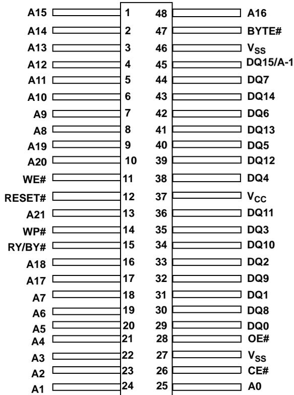
**Figure 2. UT8QNF8M8 Pinout (48)**
