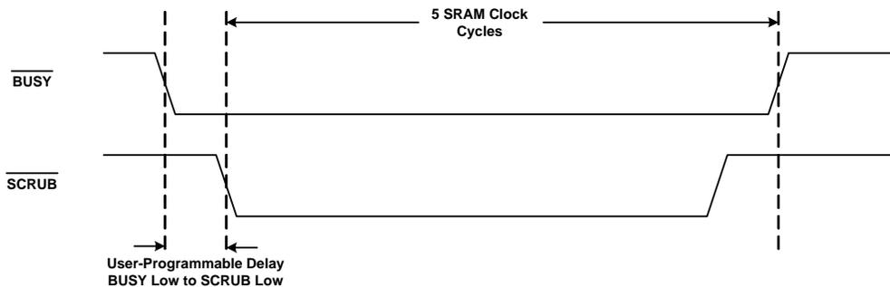
**Figure 2. Bus Timing Diagram for Scrub Signals**
