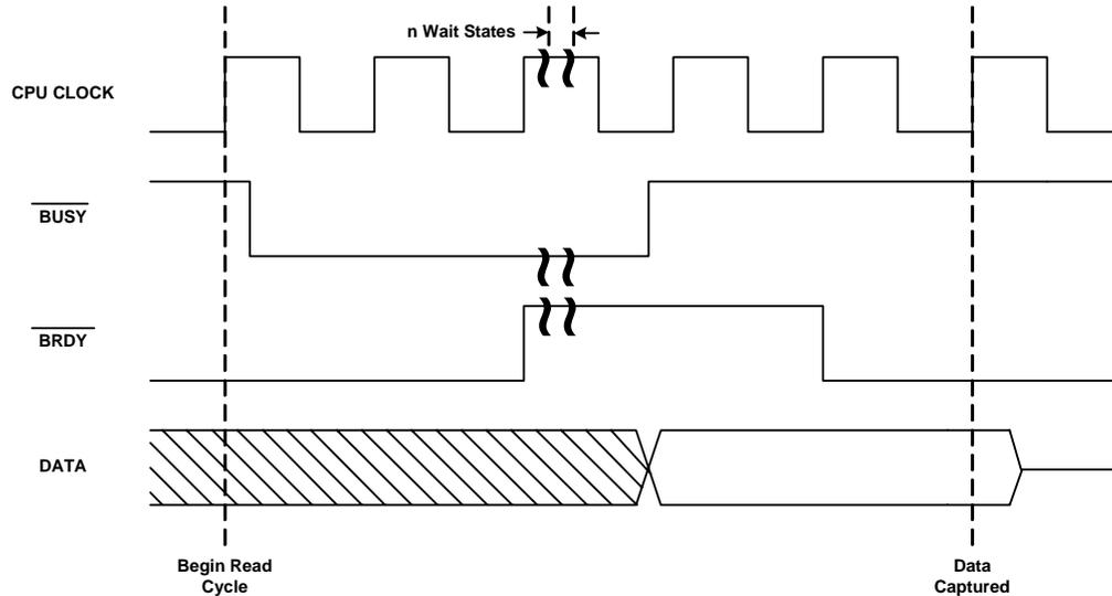
Figure 4. Typical Read or Write Timing Diagram
