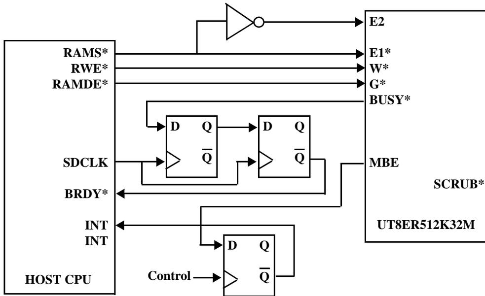
Figure 3. Master Device with Auto-Scrub and Wait-State Generation
