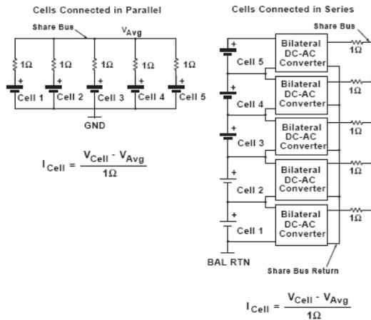
Figure 1 - Cell Balancing by Share Bus
