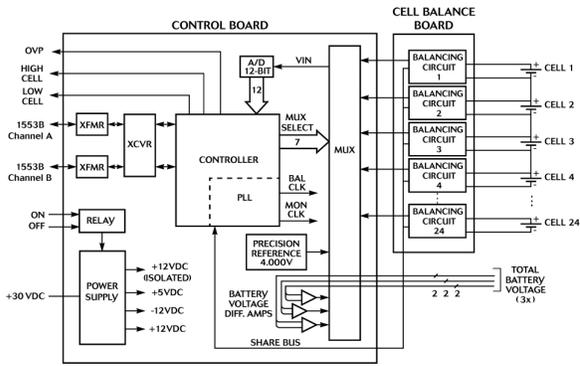
**Figure 4 - BEU Functional Block Diagram (Single Channel)**
