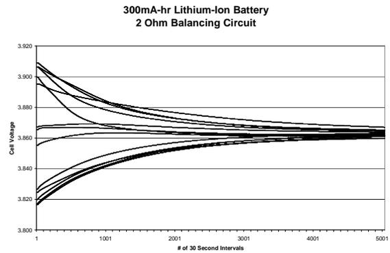
Figure 9 - Balancing of 13 Cell Battery
